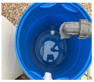
• **Sump**: This is the container placed under the media based grow bed to collect the water and pump it back to the fish tank.
