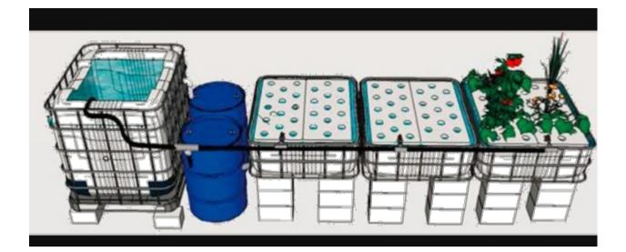
• Media-based aquaponics - In this system, plants are grown in a media-filled bed or container, with water circulated from a fish tank through the bed. The media, such as gravel or clay pebbles, provides a surface area for beneficial bacteria to colonize, which helps to break down fish waste and maintain water quality.
